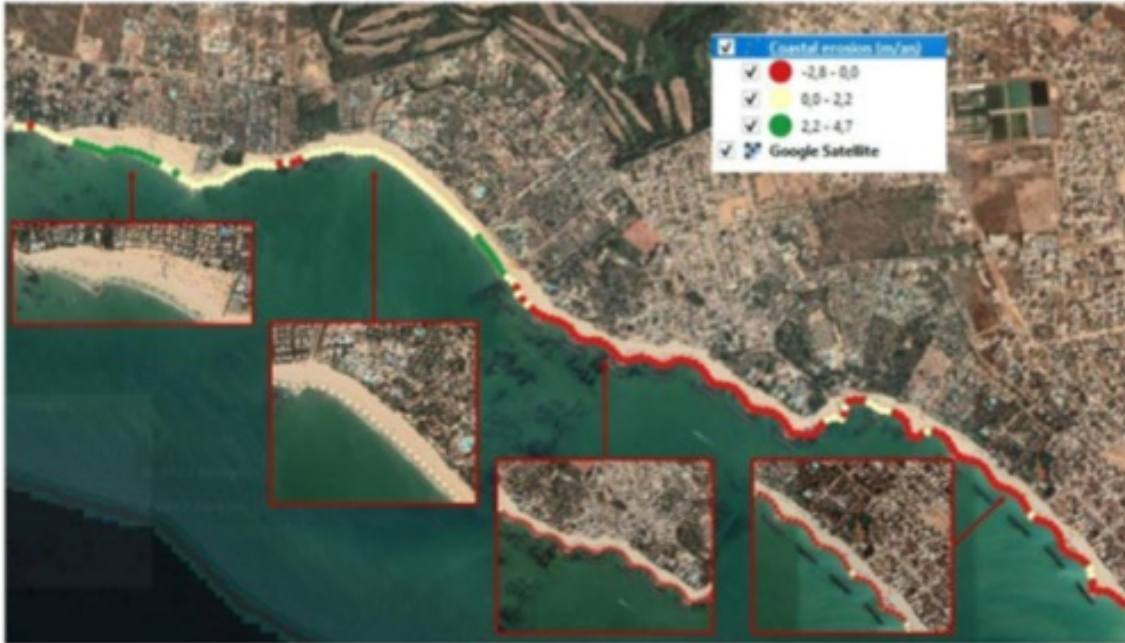
Annual evolution of coastal erosion in Saly Portudal between 2002 and 2021. Some areas have suffered a decline and others, an accretion. Recent construction work on the breakwaters is said to have contributed to the reduction of coastal erosion.
